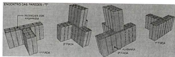
EXECUTAR EM TODOS OS ENCONTROS DAS PAREDES ATÉ A VIGA DE RESPALDO E NOS OITÕES ATÉ A TERÇA.
